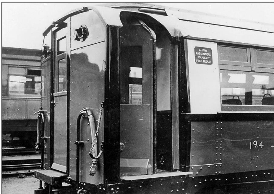
Figure 3: Close-up of the enclosed end of Hampstead gate stock Car No.194 showing the revolving door trial proposed by W.S. Graff-Baker. Only this single door position was fitted with this type of doorway. All the other doors were of the conventional sliding type. The position of the door engine is not indicated in this photo, nor in the general arrangement drawing of the vehicle. Photo: LT Museum.
