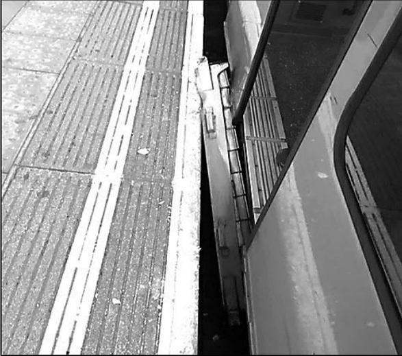
At 15.30, an outer rail Central Line train entering service from Hainault Depot was found to have smoke coming from underneath it and on arrival in the platform, a dislodged battery became wedged between the platform, train and track (*Left*). There was some damage to the train and also the platform edge. The train was worked to depot at 18.25 and the outer rail platform remained out of use for the rest of the day because the platform edge had been damaged.
