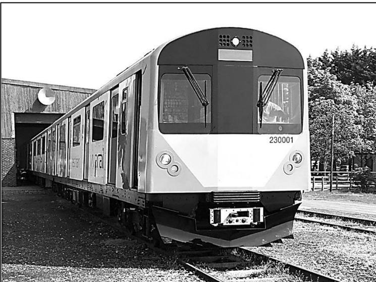
The Class 230 (*Left*) has been designed as a cost-effective solution to over-crowding on the rail network. The train costs considerably less to acquire and run, about a third less than a comparable unit, and uses about a third less fuel. The ground-breaking engine modules allow the train to be maintained trackside, rather than needing to return to a depot.
