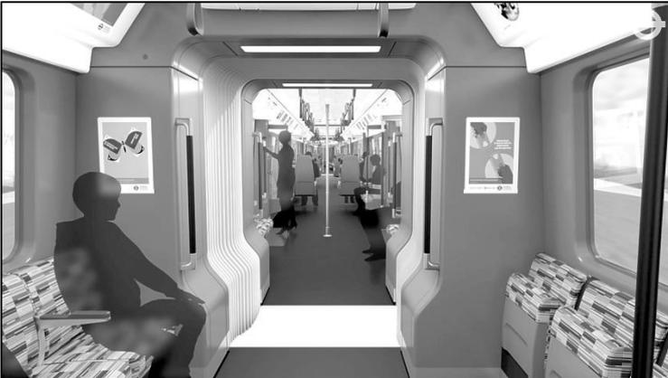
Images of the future class 345 Aventras trains for Crossrail, being built by Bombardier in Derby, showing the exterior (*Above, Left*), the seating arrangements (*Above*) and the 'walk-through' feature (*Left*). Each train will provide space for 1,500 passengers in nine fully-interconnected, walk-through carriages. At over 200 metres in length, they are over one and a half times longer than the longest Underground train.
