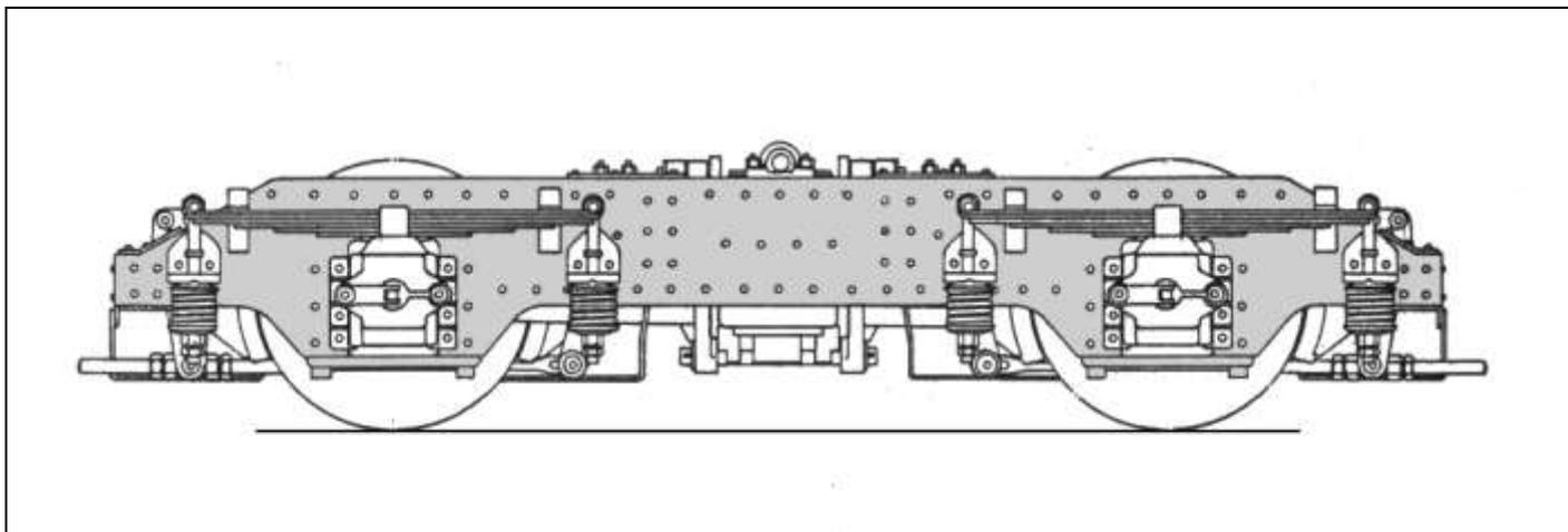
*Fig. 4: District Railway K2 Type bogie. This became the standard bogie for the District up to 1935 and was later successful enough to be used to replace bogies on some Metropolitan Railway vehicles. The design was standard British, with steel plate side frames and leaf spring primary suspension. It was designed to be used with 2ft 6in or 3ft 0in wheels.*
