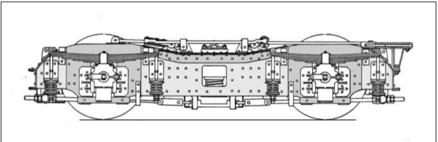
*Fig. 2: The new District motor bogie known as the A2 Type with a wheelbase of 7ft 10ins and 36 inch motor wheels. The bogie was designed with a conventional steel plate frame but strengthened as shown in the drawing by the darker areas. This bogie became last District design and was ordered for all new motor cars built up to 1936. The bogie, like most of this era, was "handed" to allow it to be connected to the brake rigging at the inside end – the right hand end on this drawing.*
