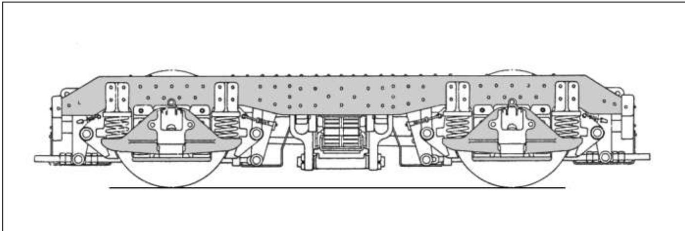
*Fig. 3: The prototype trailer bogie designed in 1922 as a replacement for the old cast steel bogies. The bogie had a conventional steel plate frame but steel coil primary suspension and leaf bolster springs. The primary suspension looks a bit like the BR B4 design of 1963 but it wasn't adopted by the District in 1922, probably because of the light frame. Only one example of it was built and it was put under B Stock motor car No.16, together with the first A2 motor bogie.*
