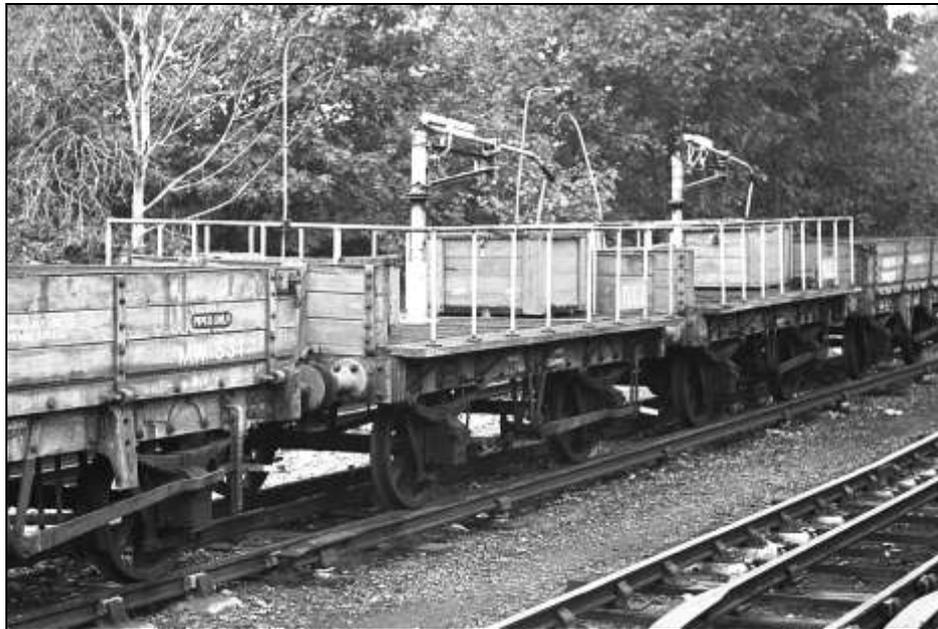
**Left:** The two Tunnel (Telephone) Line Cleaning wagons TLC1 and TLC2 are seen in Ealing Common 'Alps' depot sidings shortly before being scrapped. They were converted in June 1948 from Metropolitan Railway Ballast Wagons – TLC1 from BW108 (built 1904) and TLC2 from BW248 (1893). After being stored out of use for some years they were cut up on site at Ealing Common on 16 September 1978 by Cashmores.
