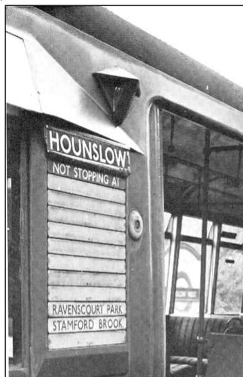
Fig. 15: Door fault indicator light as tried on the centre-guard train in 1949. This photo also shows the new type of destination plate introduced on stock built from 1938 for the non-stop indicators. Non-stop indicators were abandoned from January 1951. Photo: LT Museum.
