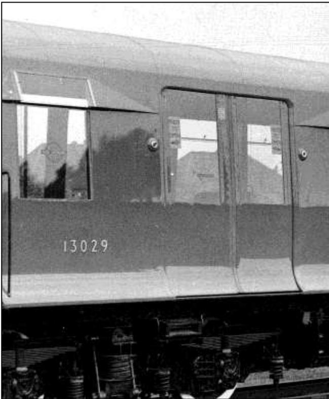
*Fig. 1: Part of O Stock motor car showing the door glazing slightly offset (by almost an inch) in one door. Photo: LT Museum.*
