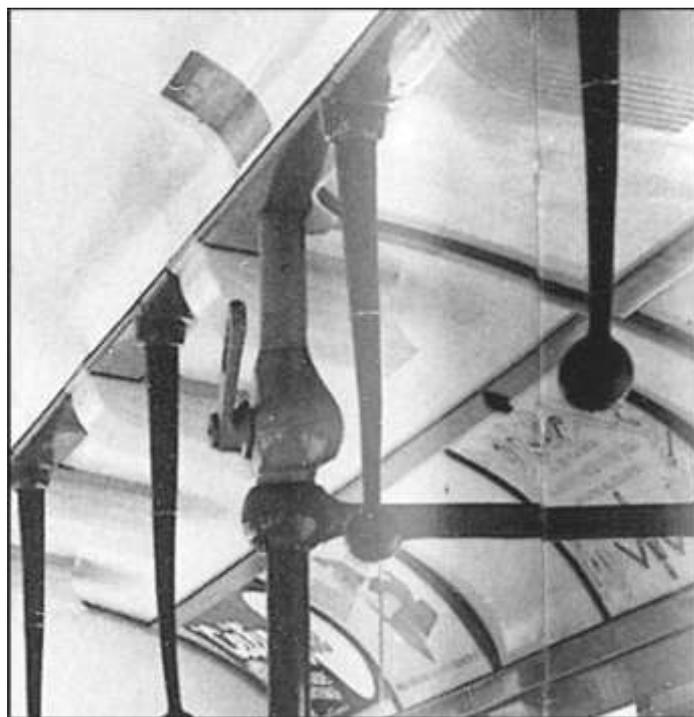
*Fig. 8: Lever type of pull-down passenger emergency valve as used on P & Q Stocks. Photo: LT Museum*
