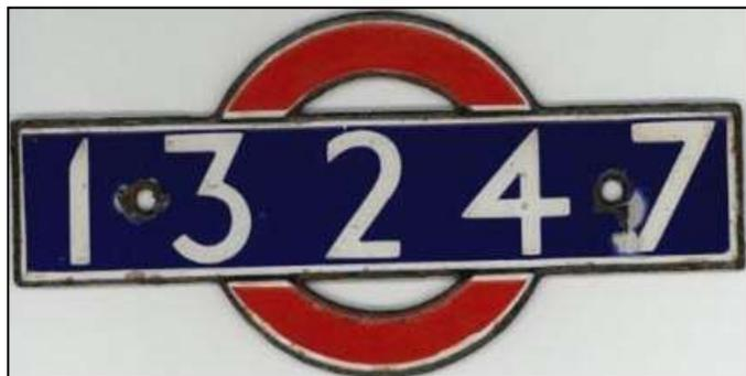
*Fig. 9 (Left): O Stock interior number plate as used on the "D" or 140xx cars. It was screwed to the ventilator grille over the end doors. The "A" cars had no grilles and the numbers inside the cars were transfers.*
