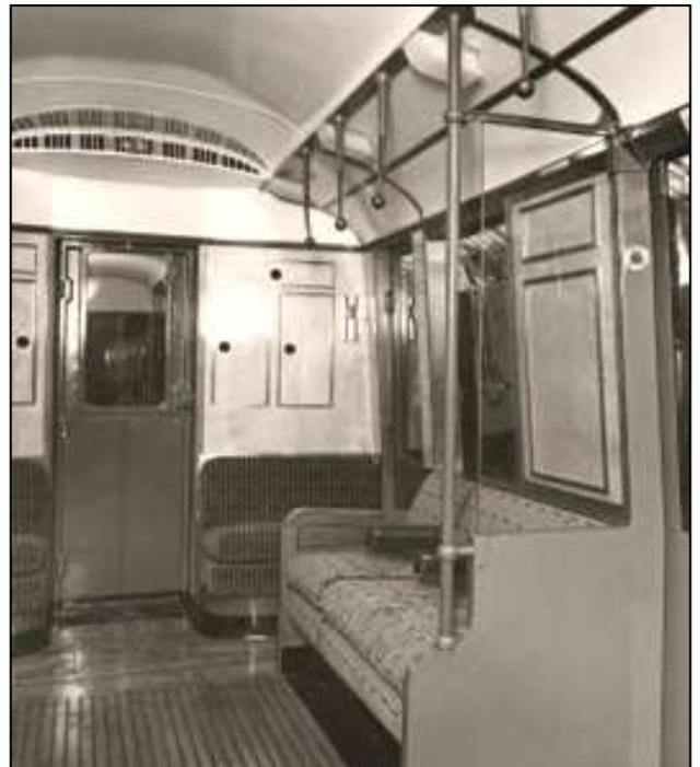
*Fig. 5: Ventilation grille on trailing end of a Q Stock trailer. This is the dummy cab end. Photo: LT Museum*
