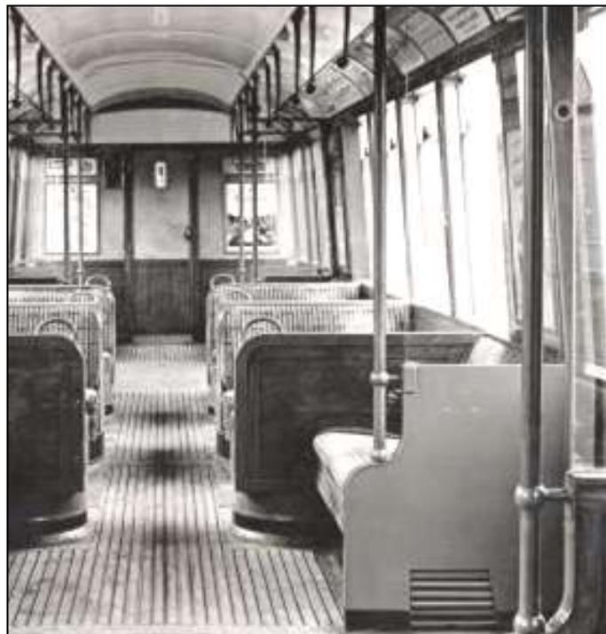
*Fig. 6: Interior of P Stock "A" motor car showing Metadyne ventilation grille at the base of the draught screen. Photo: LT Museum*
