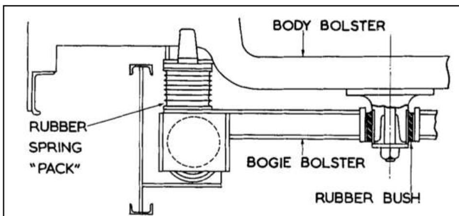
*Figure 4: Diagram of rubber suspension units that replace the steel side rollers and centre bearing on the 1967 Tube Stock. The rubber side bearers carried the car body weight. They were flexible enough to allow the bogie to turn up to six degrees from the centre.*
