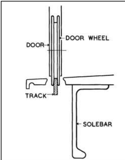
Figure 2: Diagram showing the arrangement of the solebar and door track for 1967 Tube Stock. Drawing, Webster (1969).
