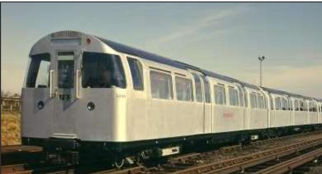
Figure 3: Official photo of 1967 Tube Stock 4-car unit showing the original cab front, ventilation slots above the windows and the curved door glazing. The body was unpainted, sanded aluminium and the roof black. The photo was most likely taken in December 1967, shortly after this unit (3006) was delivered to Ruislip Depot. Photo: LT Museum.
