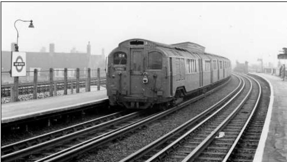
The example (*left*) of the 1923 build at East Acton shows pull-down saloon windows instead of tilting quarter lights, steel sheet doors instead of ribbed, and the guard’s door stopping short of the clerestory roof line. However, this car does have triangular vent scoops, which suggests it may have been a prototype for the 1924 and 1925 batches, but nevertheless, it is definitely a 1923!
