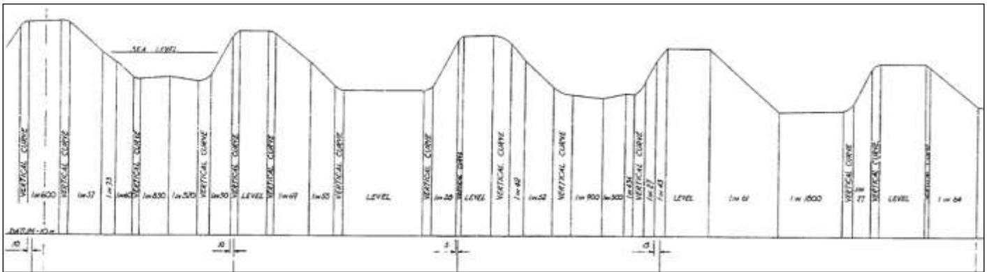
Figure 2: Section of gradient profile of westbound Central Line between British Museum (now closed) and Marble Arch showing the "sawtooth" profile with nominally 1 in 60 approach gradients and 1 in 30 exit gradients. The actual gradients were often steeper. Source: LT Chief Civil Engineer's drawing.
