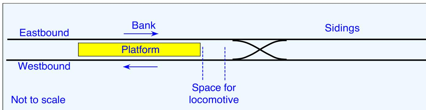
Figure 7: Schematic of the track layout at Bank, CLR, 1900, based on a signalling plan prepared as part of a bid by Westinghouse for the signalling of the line, dated 10 March 1899. The space to the east of the westbound platform allowed a locomotive to stand between the platform and the crossover. The original Westinghouse diagram shows a shunt signal was to be provided at the east end of this space to allow the locomotive access into the sidings to couple to a train therein. Diagram: Author.
