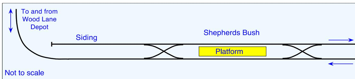
Figure 8: Schematic of the track layout at Shepherd's Bush, 1900. The station has a crossover at each end of the platforms. One of the tracks is extended beyond the siding to become the access track for the depot at Wood Lane. Diagram: Author.
