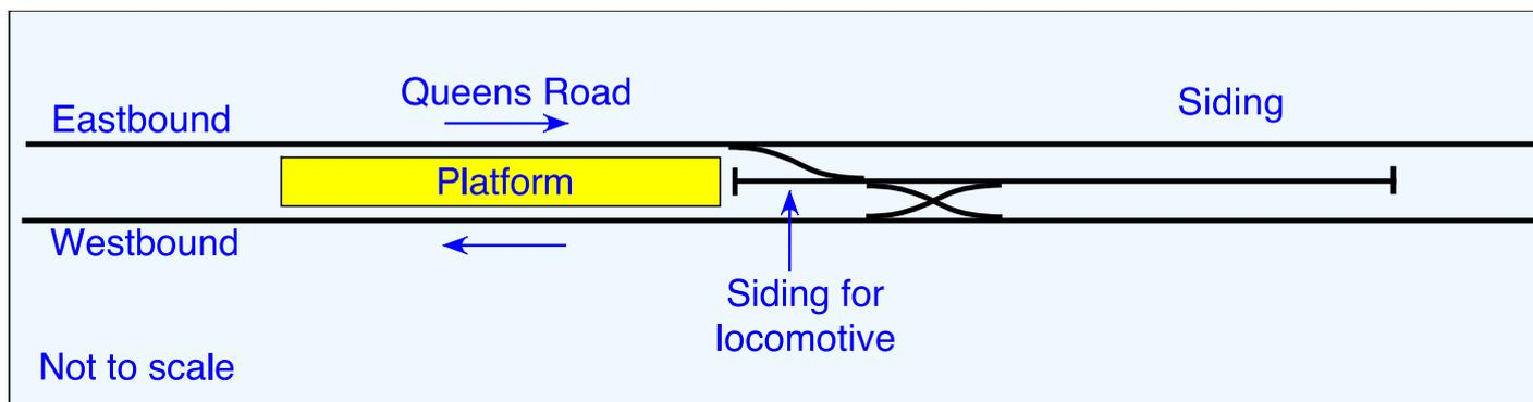
Figure 10: Schematic of a Central London Railway reversing siding as built at Queens Road (now Queensway). The arrangement was repeated at British Museum and Marble Arch. Unlike the terminals, a dedicated locomotive siding was provided. The sidings at Marble Arch and British Museum survive today but the one at Queens Road was taken out of commission on 12 July 1982. Diagram: Author.
