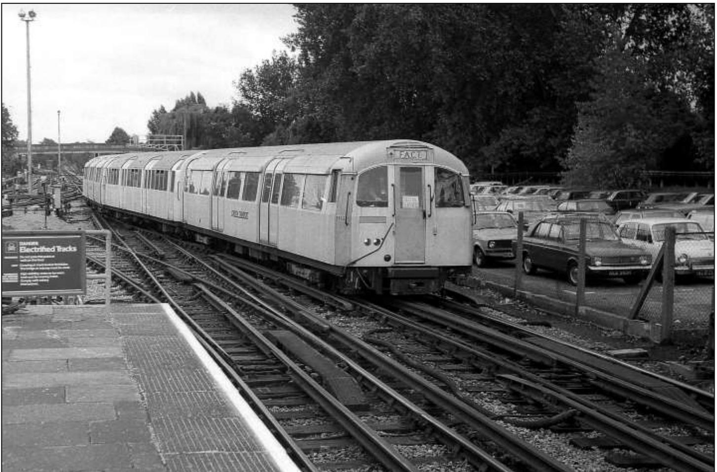
**Previous Page:** (Lower) A three-car unit of 1960 Tube Stock has departed the siding west of Woodford and is proceeding across the crossover onto the eastbound line. This train was the one that was used for the Fully Automatic Control of Trains (FACT – seen in the destination box) which, although successful in its own way, was abandoned because of financial reasons.
