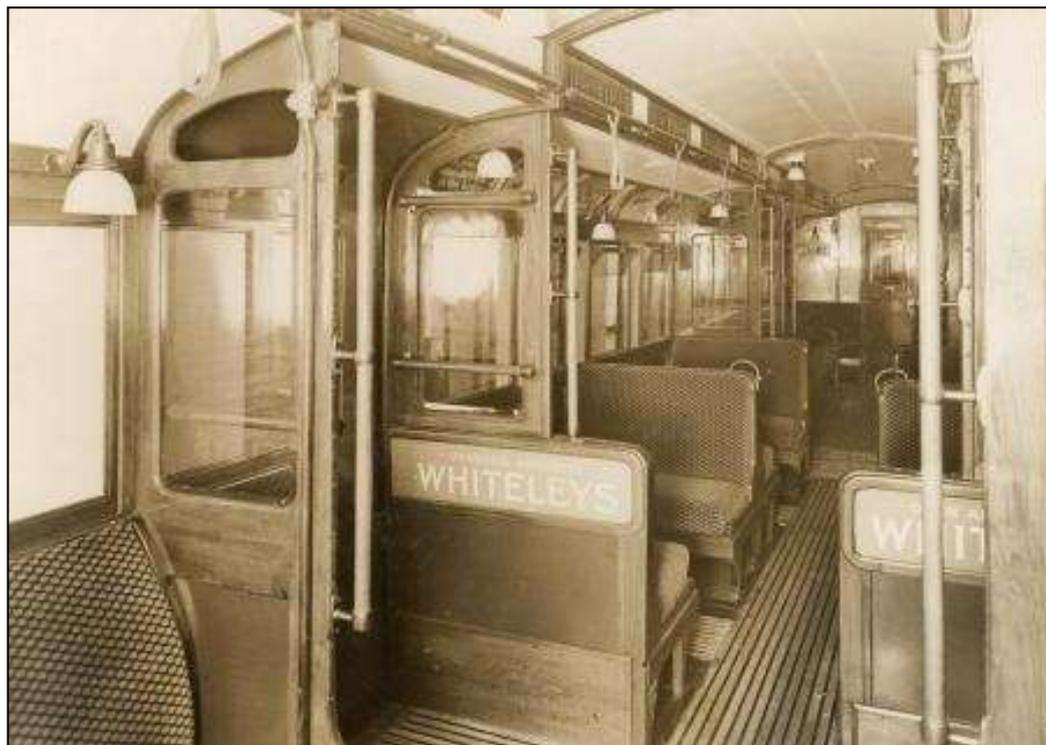
*Figure 5: Interior of CLR trailer car No.40 after conversion to air doors in 1925, showing the transverse seating between the two doorways. The interior finish shows a close similarity to other Underground vehicles built around this time, both Standard tube stock and the District’s 1923 G Stock. The lighting has been rearranged with shaded bulbs scattered around the seating areas. Only the doorways have lamps at ceiling level. Photo: LT Museum.*
