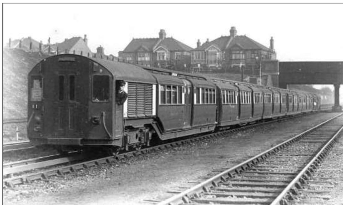
*Figure 7: CLR train of Ealing Stock is approaching the Ealing Broadway terminus next to the GWR. The leading car is a 1915-built Brush motor car showing the new, wooden body it acquired as a result of its conversion to air doors. It has the G type bogies that were fitted when it worked on the Watford line. It still has the axlebox mounted shoebeam brackets it needed on that line.*
