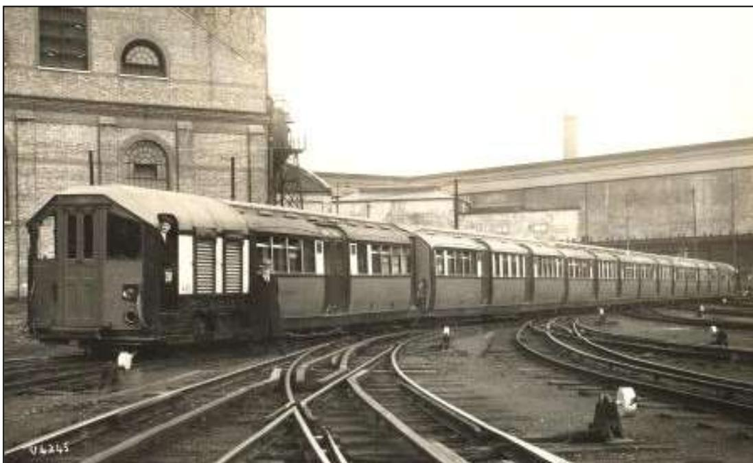
*Figure 6: A 6-car train of CLR Tunnel stock after conversion to air door operation is standing on the loop track in front of the main sheds at Wood Lane in October 1926. The train has four trailers and two motor cars. We might speculate that the manager standing in front of the leading car is Mr. Yorke himself. Photo: LT Museum*
