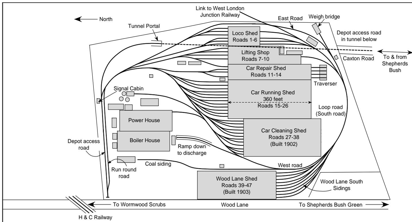
Figure 2: Wood Lane Depot in 1903 after the installation of the Wood Lane Sheds. These were added to provide the extra accommodation needed for the eight trains added with the introduction of multiple unit traction. Drawing by Author.
