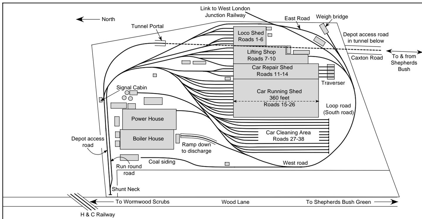
Figure 1: A plan of the CLR's Shepherd's Bush depot on Wood Lane using contemporary drawings, maps and photos. According to a sketch published in 1900, the original site did not fully front on to Wood Lane. An early Ordnance Survey map shows one or two of the original buildings still in place on the Wood Lane side of the yard. Drawing by Author.
