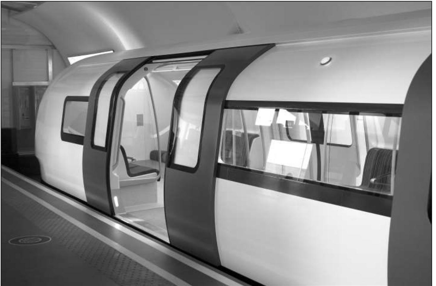
**Above:** Two views of the proposed design of the 'tube' train of the future. Interestingly, it is just possible to make out that the full-size mock-up includes a front cab door, and 'J' door between the passenger saloon and the cab. Note also (overleaf) the provision of 'walk through' between cars.
