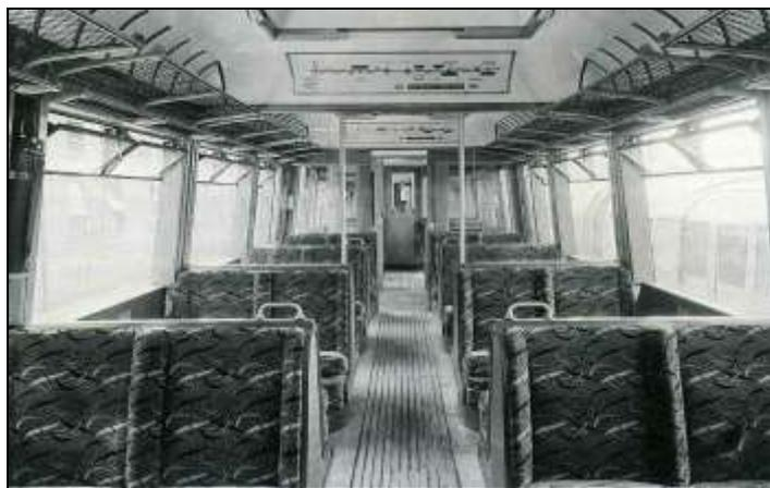
A similar feature was added to 1938 Tube Stock car 10306 at this time. A centre corridor featured with 3+2 seating and luggage racks above. A Circle Line diagram was displayed across the car for no apparent reason, but it was positioned as it was to be on the production A Stock. The front end featured curved ventilator openings above the outer windows and a six-lamp marker light display.
