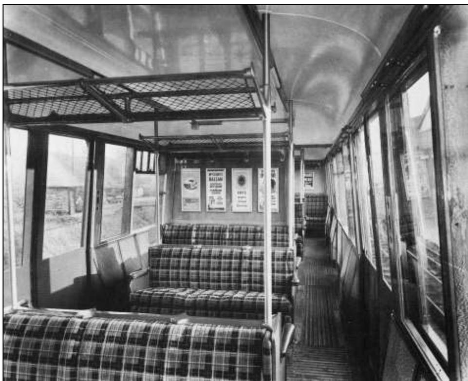
The interior layout featured a side corridor with cross-bench seating and luggage racks above (*Left*). It was later modified to a slightly off-centre corridor with 3+2 seating as car number 17001 (*Below, Left*). As 17001, the car was given a mix of high and low-back seating. In June 1947 a two-door version was completed for trials as car 20000 but had more luxurious 2+2 seating (*Below, Right*).
