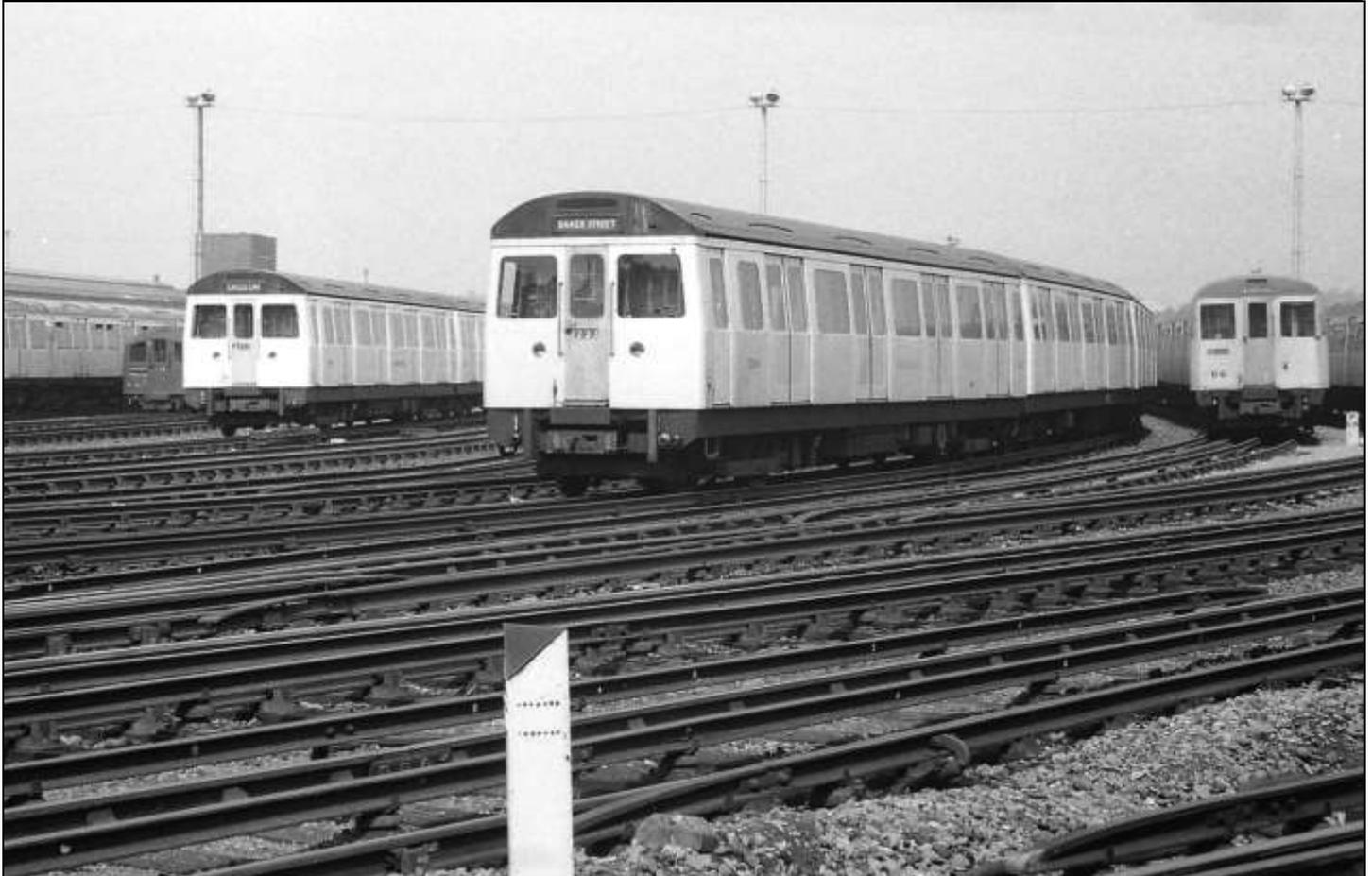
**Above:** C Stock trains stabled overnight at Neasden until June 1996 and on Sundays not all trains were required for service. Two C69 trains are seen in Neasden depot with 1938 Tube Stock on the left and A Stock on the right.
