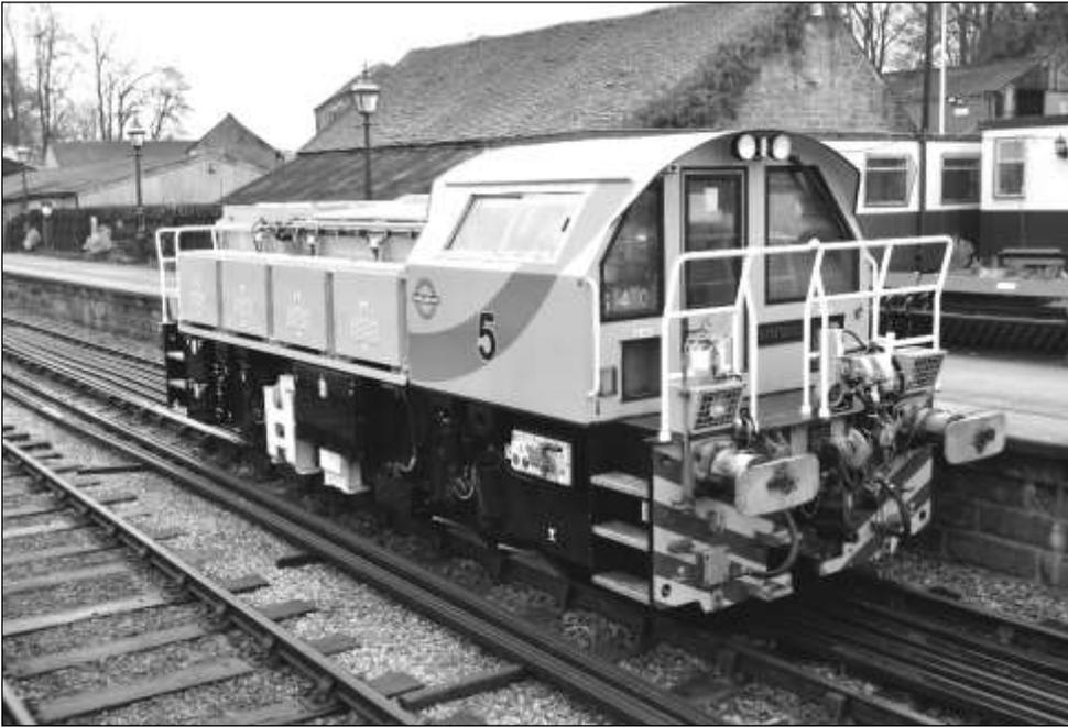
**Left:** The first Schöma diesel to be converted to a battery electric locomotive was transferred from Clayton's to the Ecclesbourne Valley Railway at Wirksworth for testing on 11 February 2015 and is seen at Wirksworth on 14 February 2015. No.5 "Sophie" has a revised livery, which includes an orange 'swirl' on the cab sides. The other three locomotives (2, 4 and 8) are still under conversion with No.2 the next. Return to Ruislip of No.5 is imminent.
