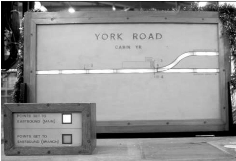
This frame was previously displayed at Covent Garden as part of the Railway Signalling display. In 2008 a number of the LT Museum Friends began restoration of the frame with a view to allowing the frame to operate as it would have done at Covent Garden. Thoughts had been given to an electronic means of 'train movement' but with the remains of the Covent Garden relay cabinets being available it was decided to use a cam timer/relay based means of demonstration. By June 2009 substantial pro-
