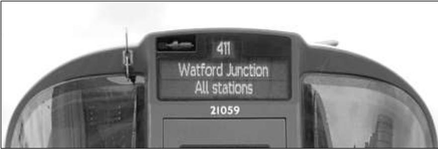
**NF 133/15** – The latest modification to S Stock is the inclusion of 'Watford Junction' on destinations in anticipation of the extension opening in 2019/20. One extra S8 train is to be provided for the extension.
