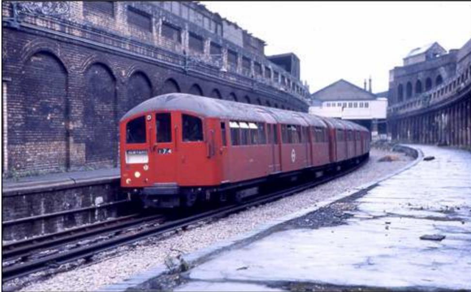
The single-line terminus at Shoreditch showing a four-car unit of 1938 Tube Stock that worked services between 1974 and 1977. The train is an EHO unit on loan from the Bakerloo Line and DM 11193 is leading.
