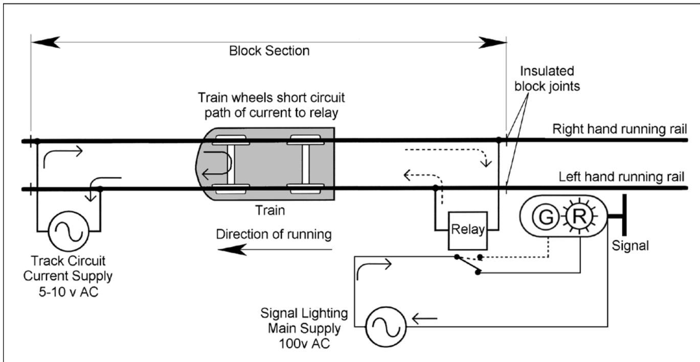
*Fig. 1: Schematic of simple track circuit showing the arrangement for automatically operating the signal protecting the section. The diagram shows the section occupied by a train and the signal at danger. If there was no train in the section, the circuits would operate as shown by the dotted lines and the signal would show a green aspect. In reality, many sections only have an insulated block joint in one rail but the principle is the same.*
