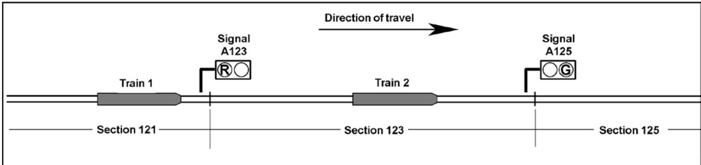
*Fig 2: Schematic showing basic automatic block signalling adopted by London Underground. A signal is provided to protect the entrance of each section. Note that automatic signals on the Underground are lettered “A” and numbered like houses in a street, odd numbers one side, even numbers the other.*
