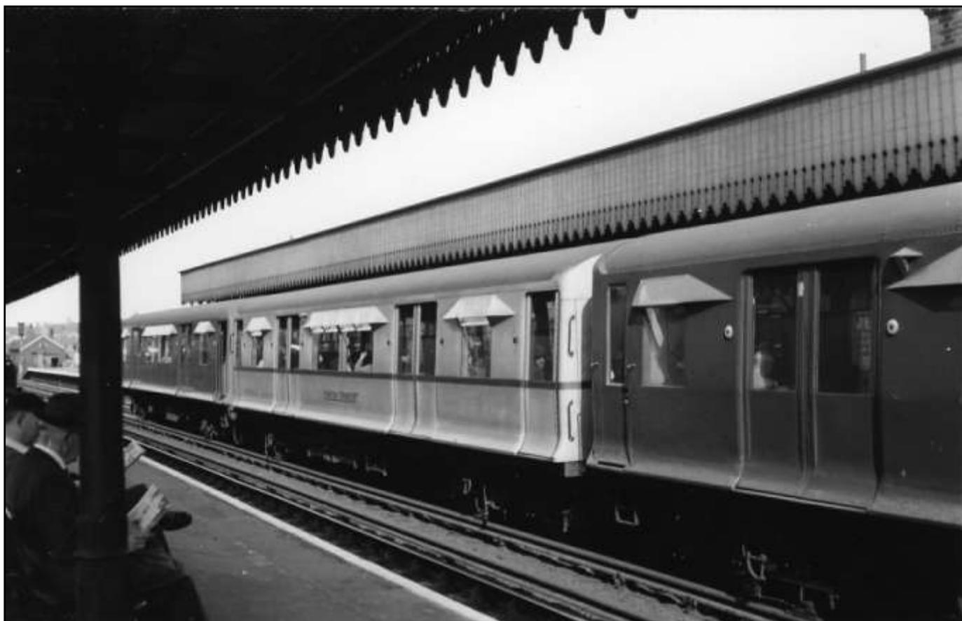
**Above:** NDM 23567 in service between red-painted R Stock cars at Wimbledon. It will be seen that the all-motored cars of R Stock didn't have wooden shoebeams when new. Instead they had bogie frame mounted shoes but had to succumb to 'conventional' shoebeams by the early-1960s.
