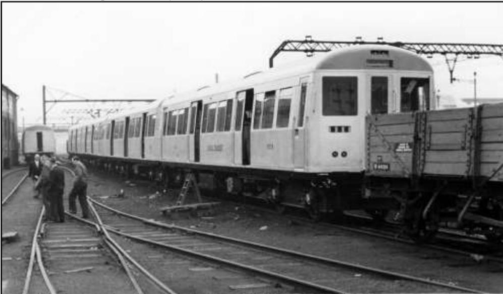
A four-car unit of A60 Stock is seen in the yard at Cravens of Sheffield, being formed up for delivery to Ruislip depot, where it arrived on 20 July 1961. Nearest the camera is DM 5028 which is now 5232 – the other end of the unit was involved in the Kilburn collision on 11 December 1984 and the best four cars were formed to make one unit.
