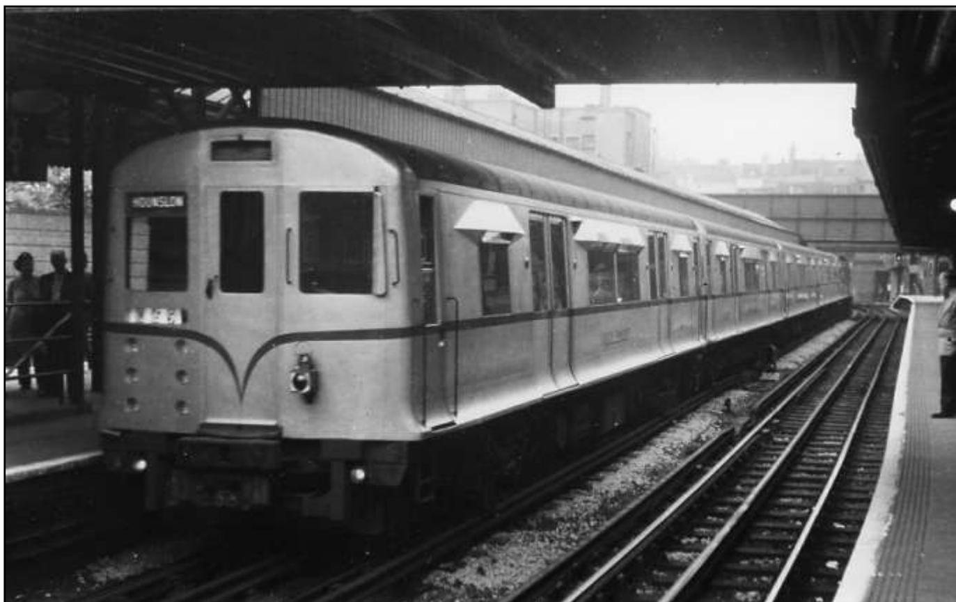
**Above:** The complete eight-car unpainted aluminium train of R49 Stock is seen at Whitechapel heading west on a rush-hour working to Hounslow West, which continued to be served by the District Line in rush hours until October 1964. This shows how the red stripe was adopted on the cab ends of DM cars, lowering slightly under the train set number box and sweeping down to form a 'V' shape. Car numbers are still in gold on the red band and were difficult to read unless you were close up!
