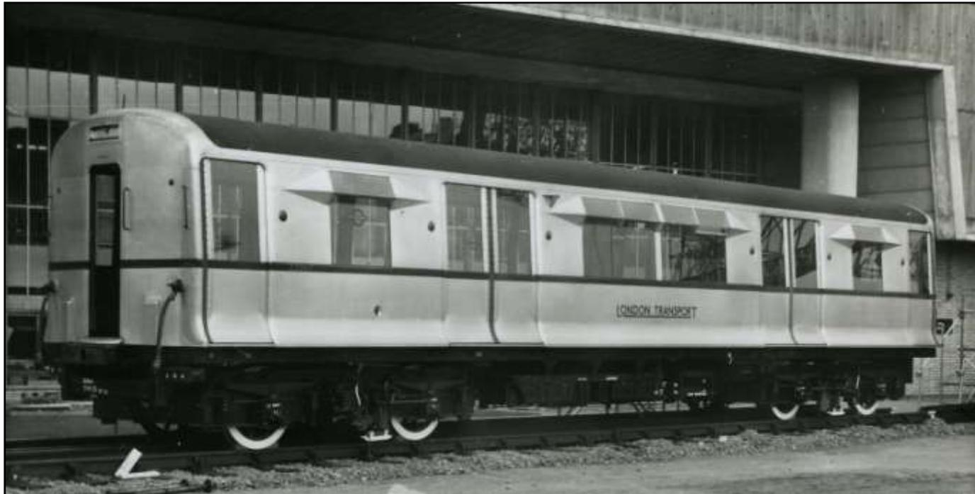
**Above:** Although the first aluminium-built R49 NDM (23231) was exhibited at the Festival of Britain exhibition in 1951, an 'aluminium' exhibition on the South Bank in 1955 saw the first unpainted car (23567) placed on show, where it is seen on 11 June 1955. The red relief came only with the waist-level stripe, the London Transport name and the red door open push buttons. The car number was in gold on the red band, close to the end single doors.
