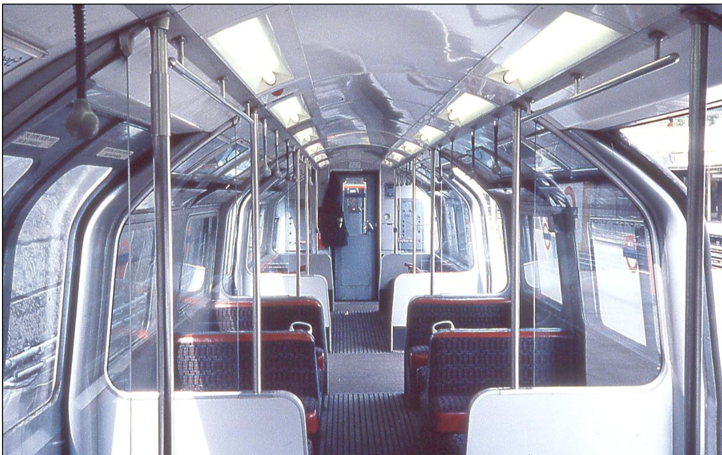
In September 1975, trailer 4209 was fitted with ceiling-mounted fans and the roof was modified to have ventilation slots for the expelled air. It is thought that this was connected with the 1973 Tube Stock, as they were built to incorporate fans from new. (Even though many of the 1973 Stock trains had been delivered, there were design and technical difficulties and it was not until October 1977 that fans were first used. However, not all cars were fitted and those that did have them were
