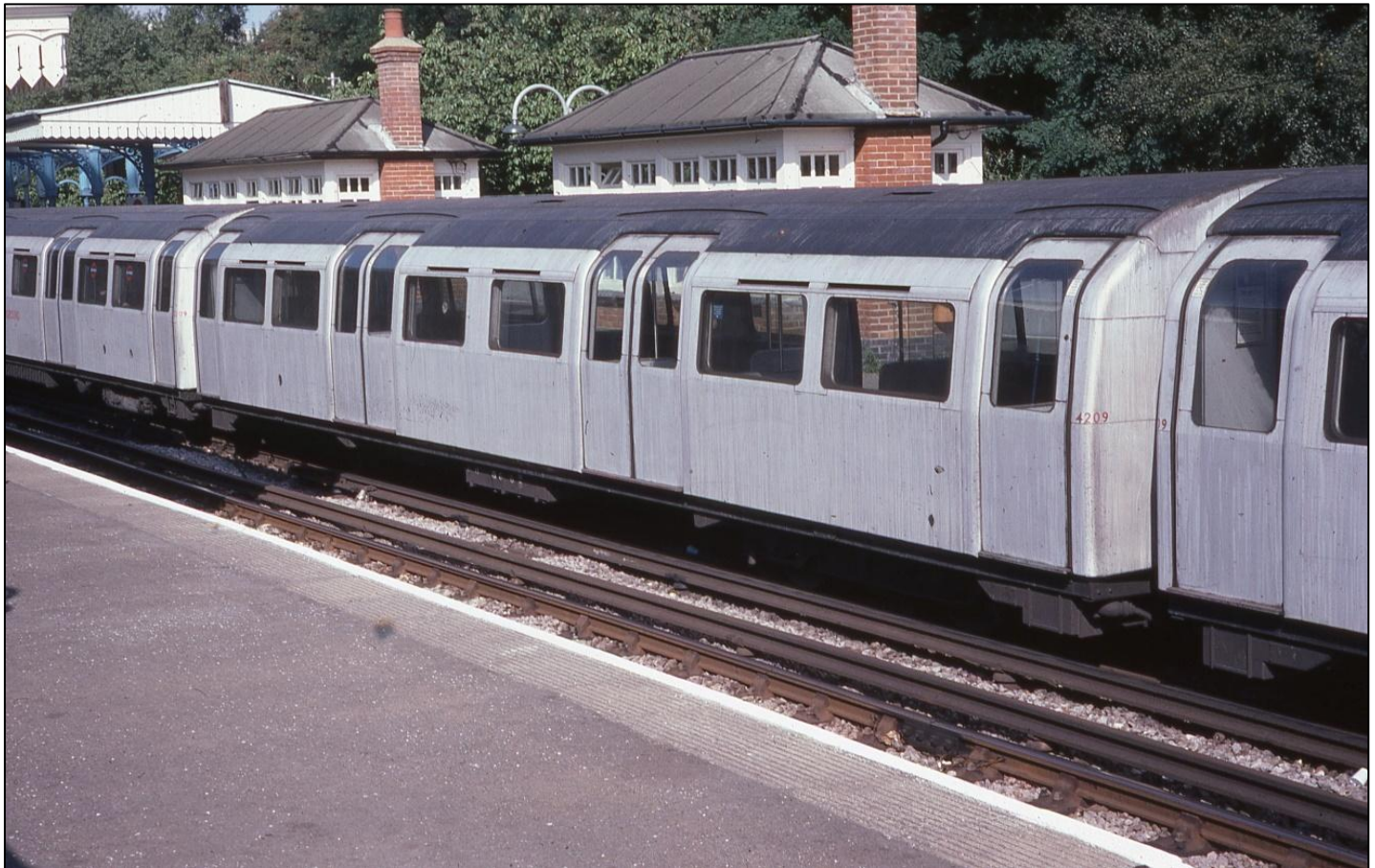
Opposite: (Lower) Trailer 4209 in platform 2 at High Barnet which was fitted with fans between September 1975 and May 1977. After the experiment ended, the slots on each side of the roof for expelled air remained.
