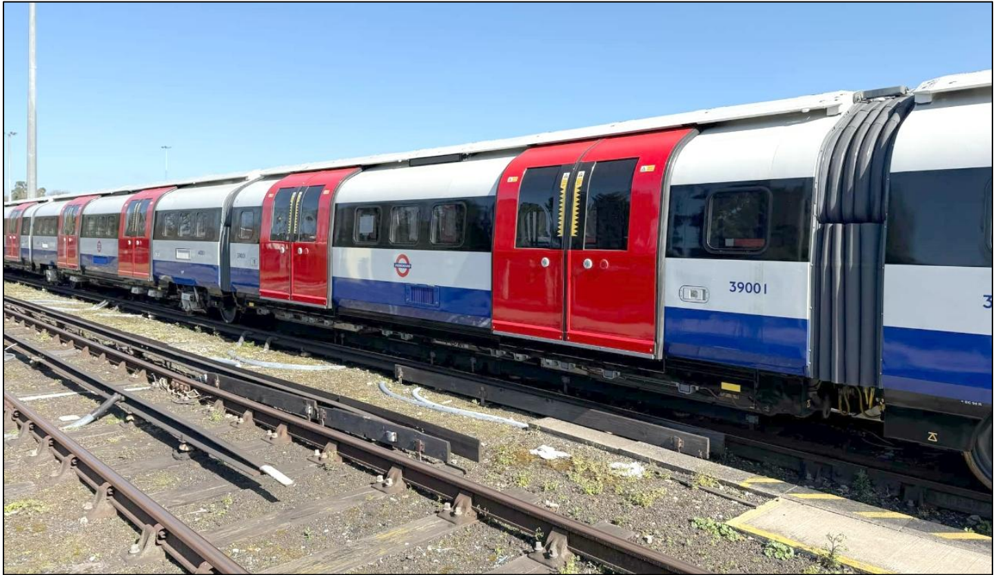
Above: One of the three 'hanging' (or 'suspended') cars in the nine-car train – i.e. bogieless, seen in Ealing Common Depot on 30 March 2025.
