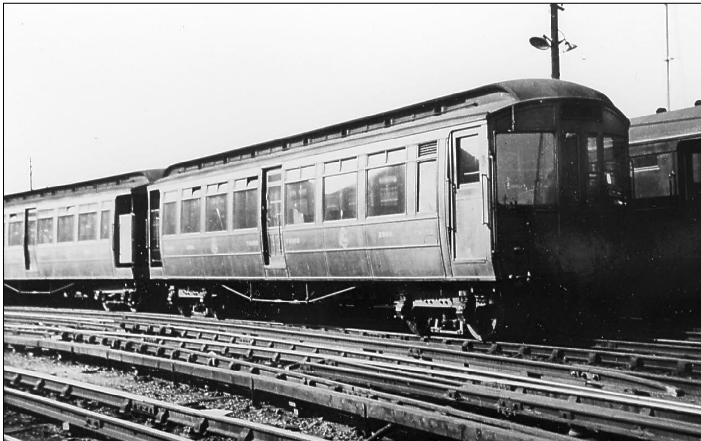
Figure 6: GN&C cars at Neasden awaiting scrapping. A single-ended wood motor car is nearest the camera with the cab end provided with proper cab doors instead of the gates originally provided. The trailing end has gates although it retains the wooden windscreen and end doors of the former cab end. The car is stripped of its shoe gear. The second car is a wood 3rd class trailer with steel plated gates. Photo: B. R. Hardy collection.
