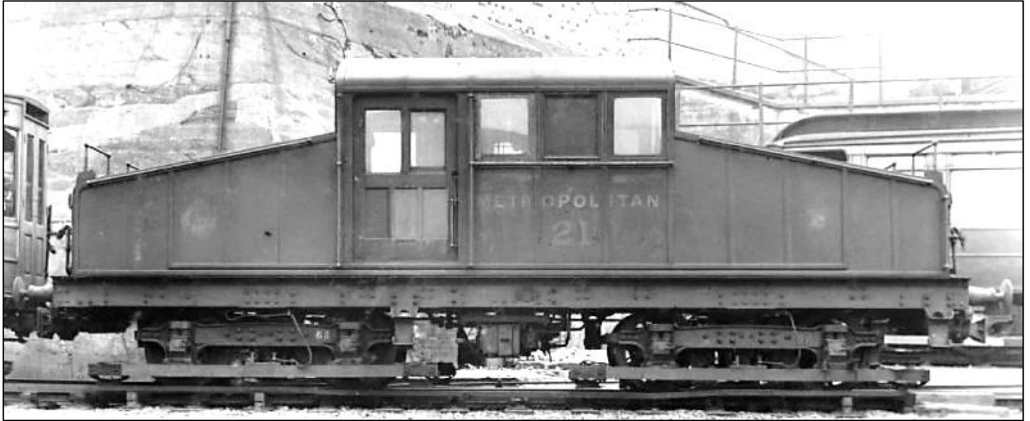
Figure 2: The replacement Drayton Park shunter No.21, ex-Metropolitan Railway 1905 loco No.1, after its conversion in 1920 to work on the GN&C as the yard shunter at Drayton Park depot. Photo: LT Museum, March
