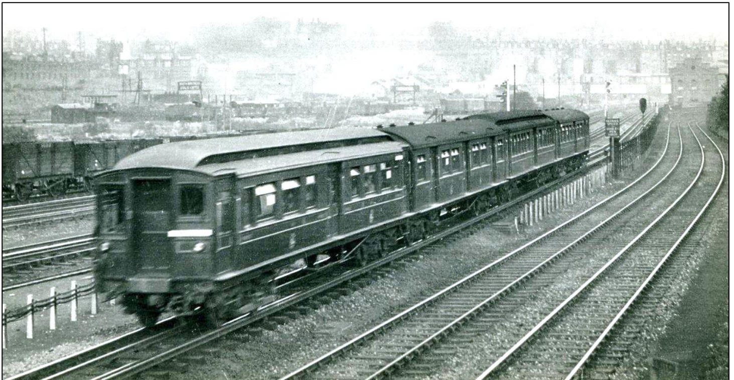
Figure 6: A 4-car set of mixed Metropolitan Railway Saloon Stock containing a complete selection of the range. The leading vehicle is a 1905 Stock driving trailer (note the asymmetrical cab window arrangement), the second car is a 1921 Stock trailer, then a 1904 Stock trailer and finally a 1913 Stock motor car. The 1913 Stock 200hp BW motor car had just about enough grunt to push a 4-car set, which was probably uncoupled from a 7-car or 8-car train at the end of the morning peak period. On 7-car trains, it was normal to run the 4-car portion at the Up end (Baker Street end) as seen here and to use this for off-peak working. Note that the driving trailer has shoe gear on the leading end. Originally, it was not thought necessary to provide shoe gear on the driving trailers. Power for lighting and heating could be obtained through the power train line provided to connect the 600-volt supply on the motor car throughout the train. On BTH trains, power for the master controller was tapped off the car lighting circuits. On BW trains, the 14-volt control power was supplied from the motor generator on the motor car via the control cable. The shoe gear was eventually added to provide an alternative contact with the current rails in case the shoes on the motor car were 'gapped'. The photo was taken some time between 1926 and 1933. Photo: Collection B.R. Hardy.
