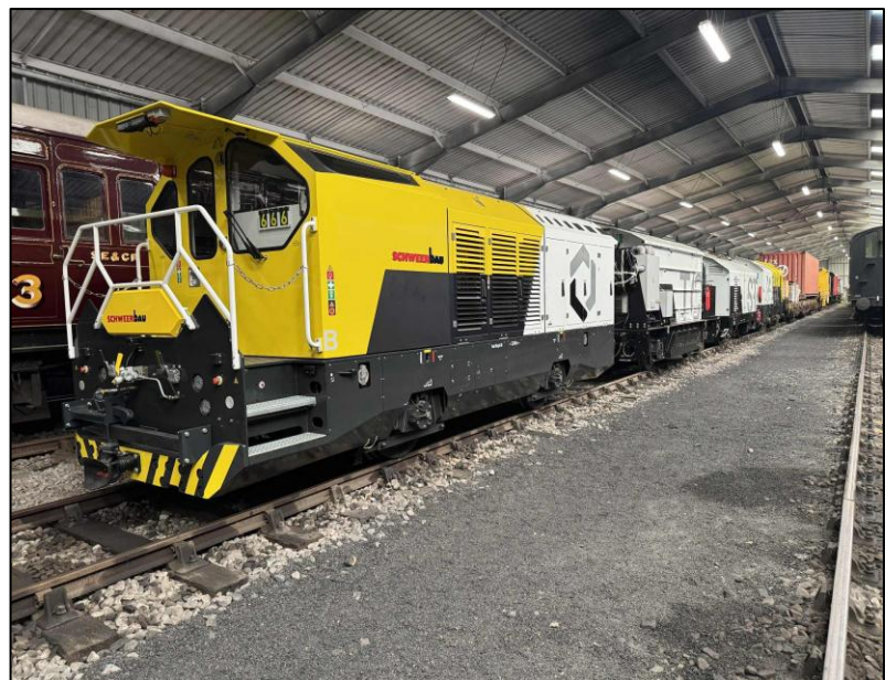
A new 4-car Schweerbau tube gauge milling and tunnel cleaning train made up of two Battery/Diesel hybrid power cars has arrived on the Kent & East Sussex Railway from Germany, along with a single car inspection/track recording vehicle. LU engineers are to do the brake testing on the K&ESR rather than on the South Ealing test track.
