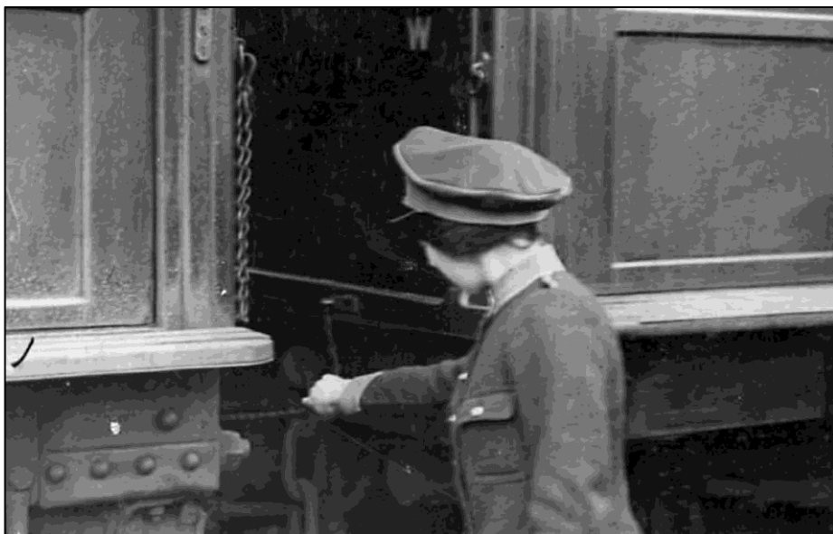
Figure 2: A Metropolitan Railway lady guard operating the uncoupling chain on a saloon stock train about 1916. Women were employed by the Met to replace men who had joined the military during the 1914-18 war. The letter W can be seen on the car end just above the lady's head. This is an early example of stock equipment identification on the Metropolitan. The W indicated BW control lines. The letter T was used for BTH control. Photo: LT Museum
