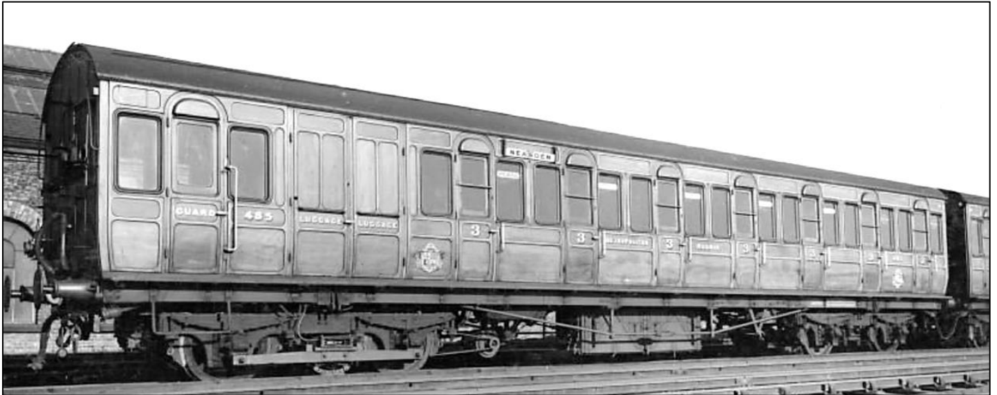
Figure 2: Metropolitan Railway 1920 Dreadnought Stock 3rd Class Brake coach No.485 in the yard at Neasden Depot. This version has a smaller luggage compartment allowing an extra passenger compartment. The shoe-gear fitted to overcome the problems with current rail gaps can be seen on the bogie at the brake end of the coach. Next along the underframe is the battery charging dynamo and then a battery box and finally a vacuum brake cylinder. Photo: LT Museum.
