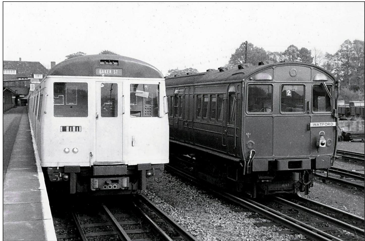
**Above:** Back in 1961, the old and the then new. On the right a train of T Stock stabled on No.24 siding, while on the left, the new order – a train of new A60 Stock, comprising one of the first three eight-car trains with black roofs, which were lost on first overhaul.
