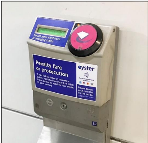
Far Left: At ungated and partially-gated stations, and at some LU/NR interchanges, Validators are provided for those using Contactless cards.
