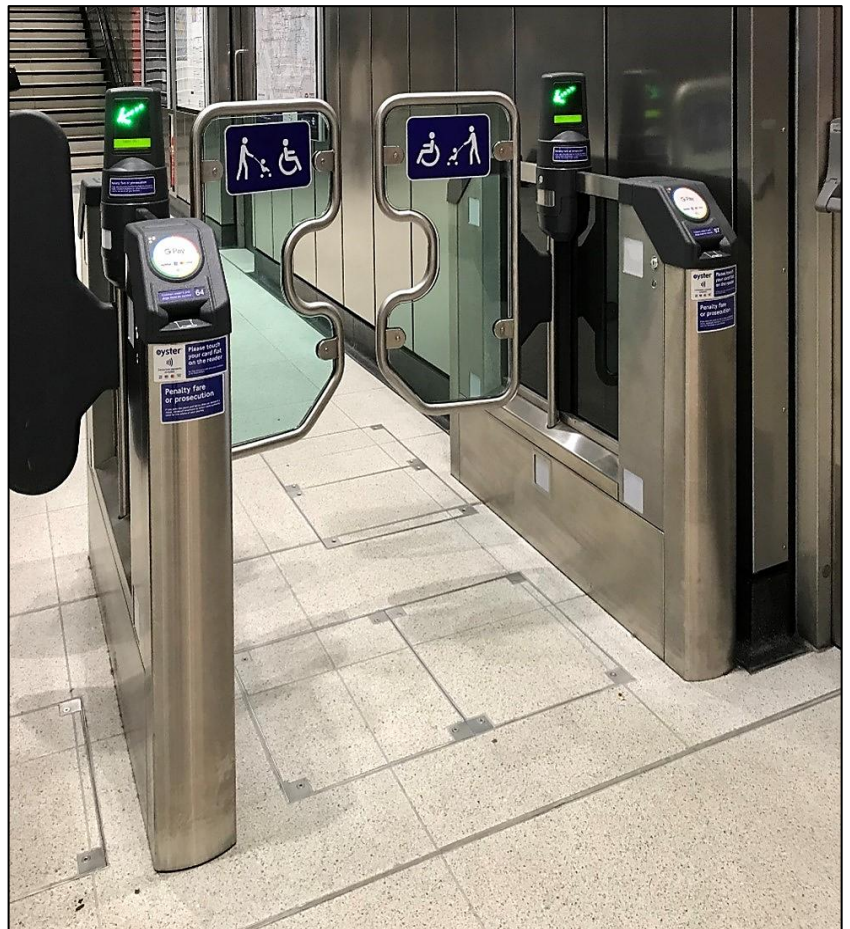
A Wide Aisle Gate in original condition at Paddington (Bakerloo) with the paddles formed of glass within a metal frame. The majority of these have since been replaced by paddles made of solid plastic.
