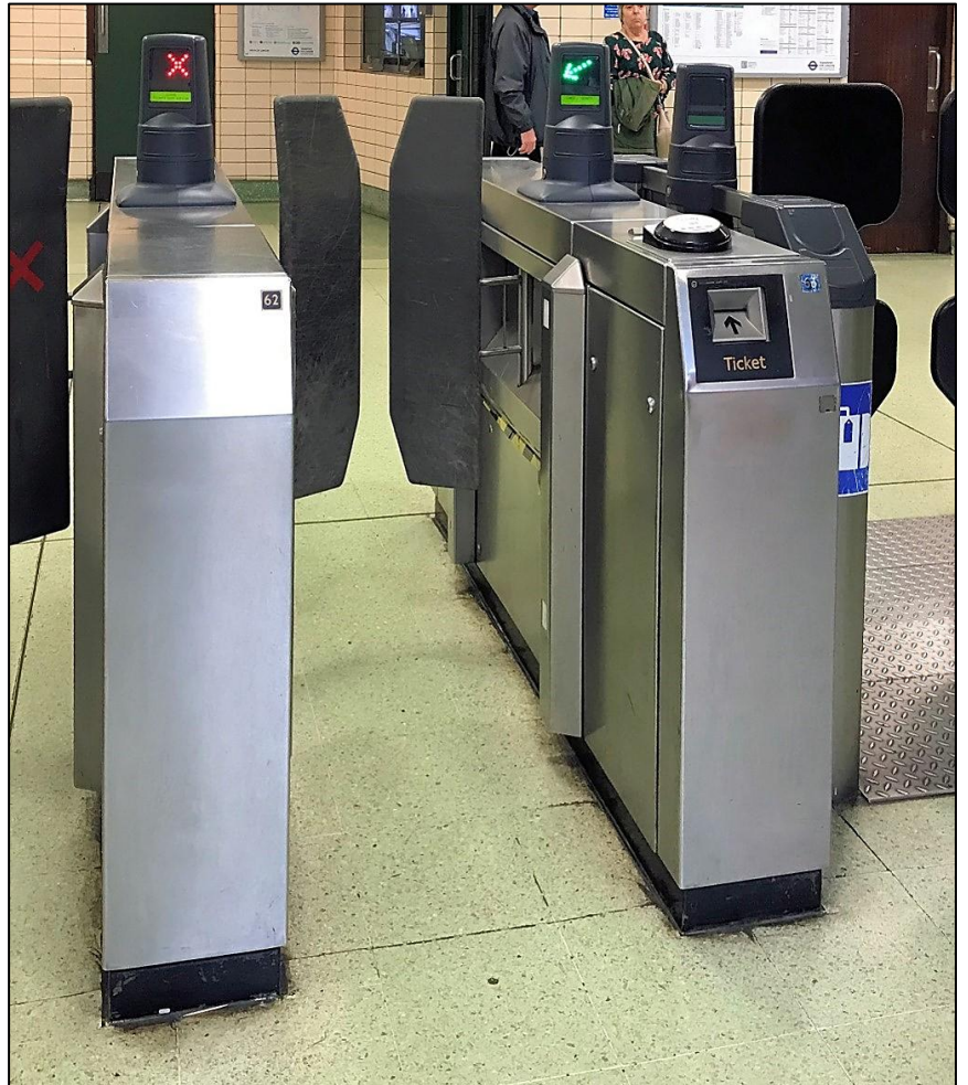
A unidirectional pneumatic P Gate configured for 'exit' at Paddington (Praed Street).
