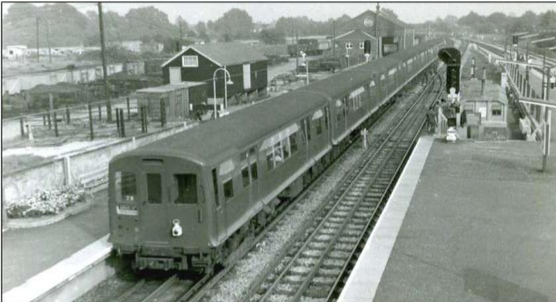
*Fig. 1: Eight-car O/P Stock train departing Amersham for Baker Street with an evening peak hour train in the early 1960s shortly after electrification was extended north from Rickmansworth. The stock was usually confined to the Uxbridge services but there were regular timetabled trips to other destinations.*
