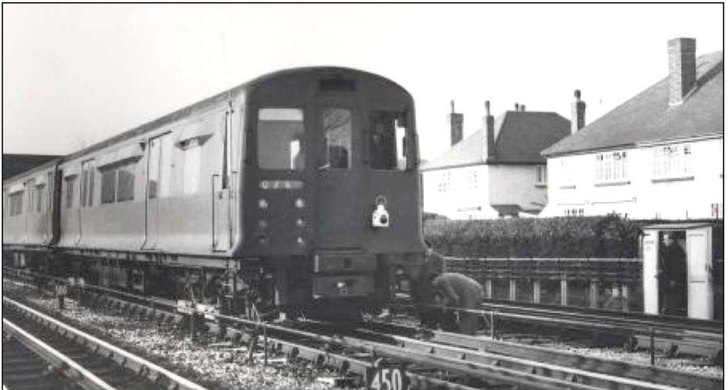
*Fig. 2: Experimental ATO train on the test track between South Ealing and Acton Town in December 1962. This is the east end car, No. 22681, which was fitted with the ATO pick-up coils under the front headstock. To the right is a temporary kiosk used to house some of the test equipment. There was another one at South Ealing station. Photo: LT Museum.*
