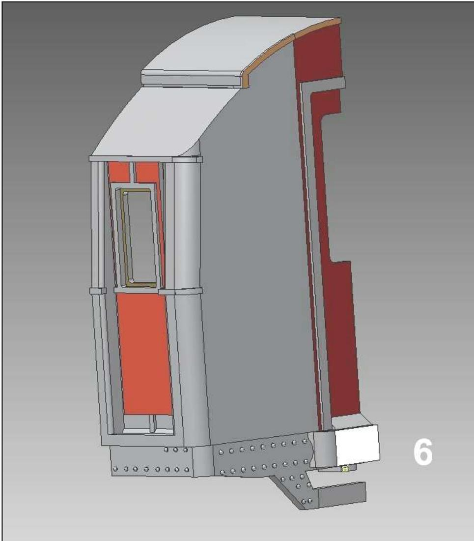
6. The front of the solebar/headstock with the ward coupler mounting, buffer and rivet pattern is visible. Half of the cab front door and the side door are pretty much complete. Similarly, at this stage, this cab could either be turned into the 1925 Cab as built or the modernised type.
