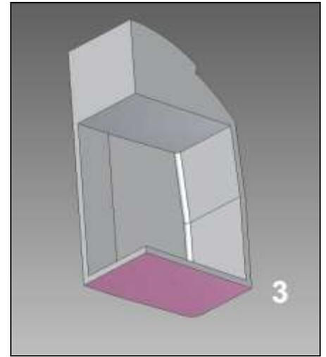
2. The floor plan sketch has been extruded to the level of the cantrail [roof eave] and the angled part of the body above the waistline created by slicing away an appropriate angled segment of the side. At the moment this is still a [virtual] solid block.
