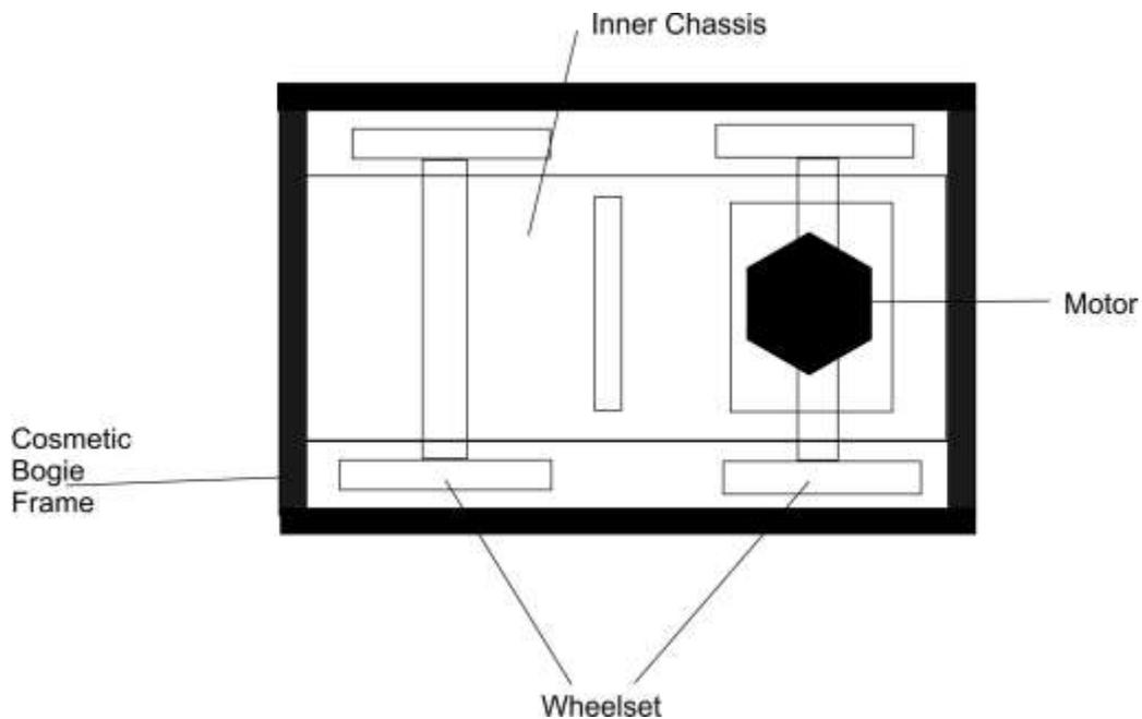
*Figure 1 – Looking Down on Conventional Motor Bogie – Outer Frame and Inner Chassis.*
