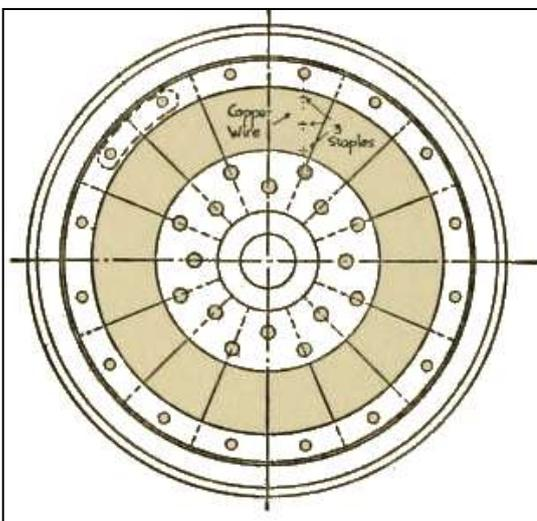
*Figure 3: Drawing of wooden centred Mansell wheel as used on Central London trailer cars.*
