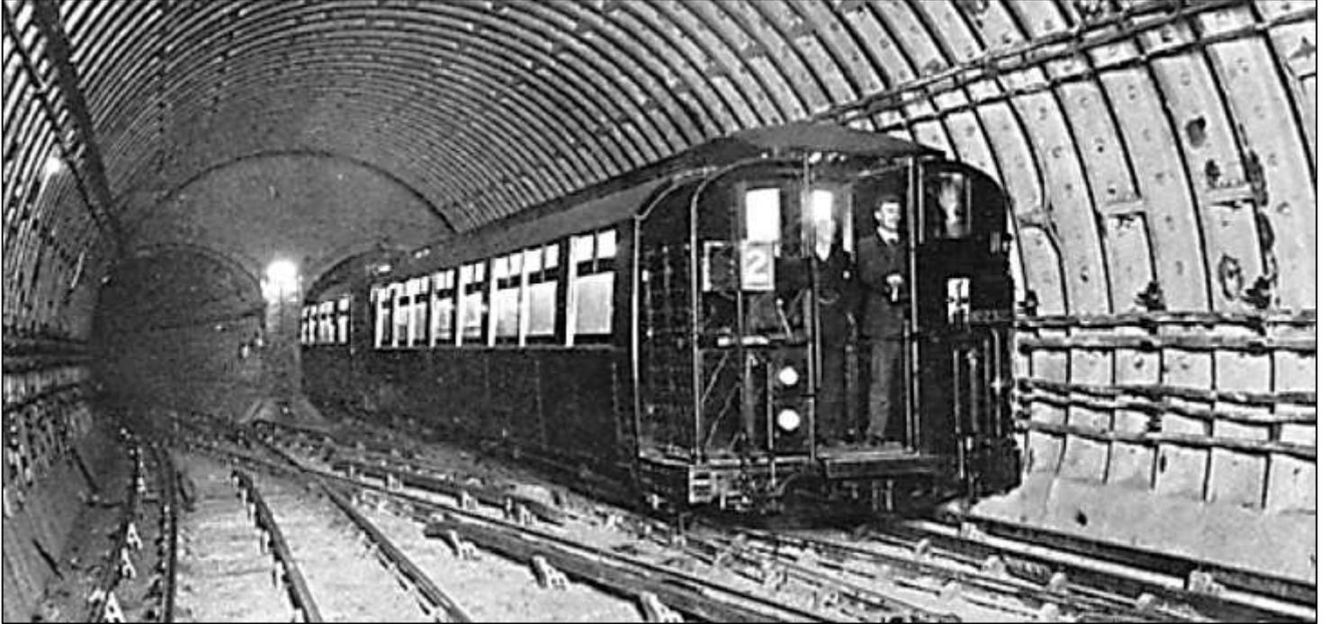
*Figure 5: LER gate stock control trailer shown in a specially posed photo at the Hampstead crossover about 1907 when the whole system was new. The driving position has a simple steel screen with a small window that forced the driver to stand whilst driving. The driver's hand is on the master controller. The platform could be used by passengers if the car was in a train where the control position was not being used. Photo: LT Museum.*
