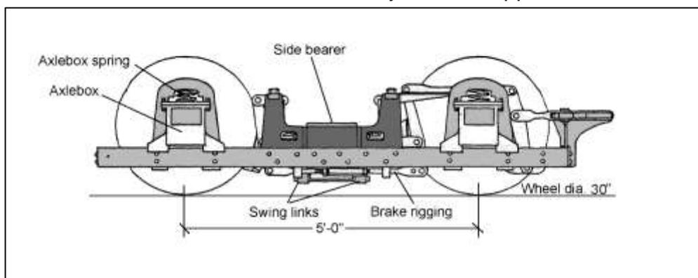
Figure 3: The LER gate stock trailer bogies were known as Type O. This tiny lightweight bogie survived for the life of the stock but it does not appear to have been provided with any secondary suspension. The drawing was adapted by the author from one by the late Stuart Harris.
