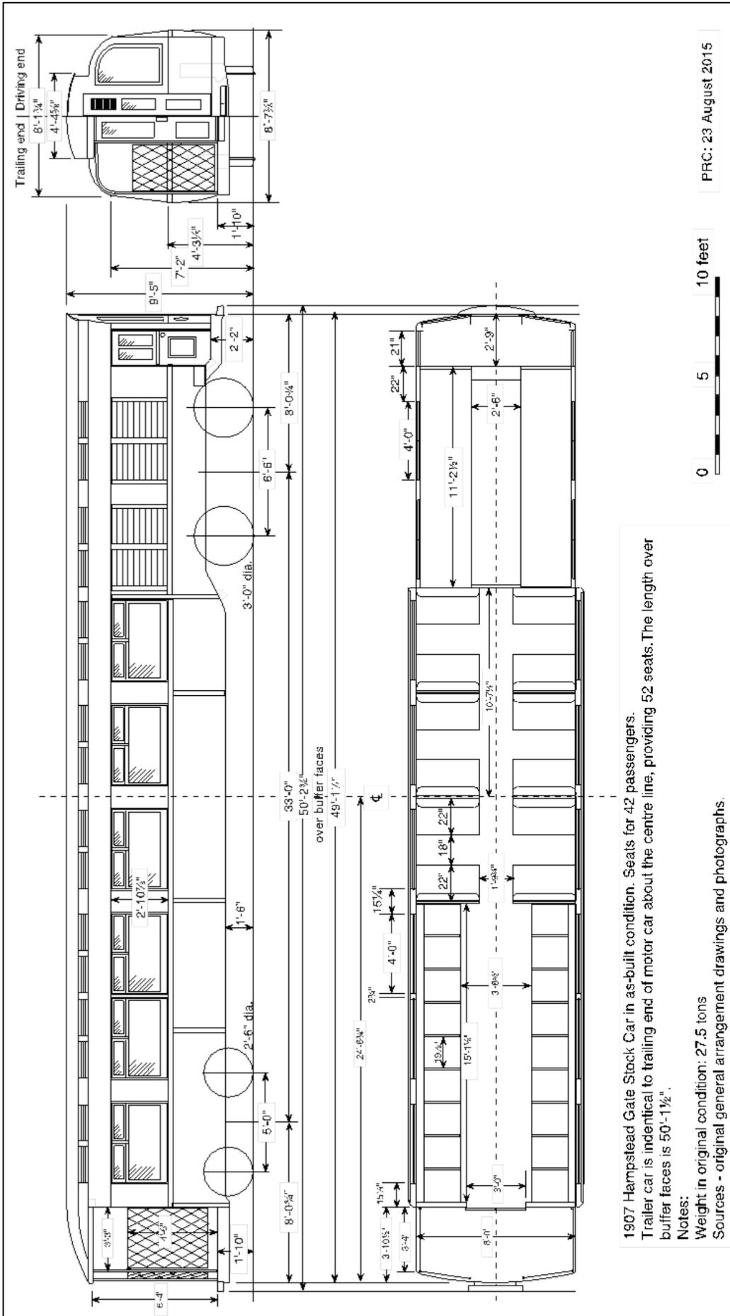
1907 Hampstead Gate Stock Car in as-built condition. Seats for 42 passengers. Trailer car is identical to trailing end of motor car about the centre line, providing 52 seats. The length over buffer faces is 50'-1 1/2".
