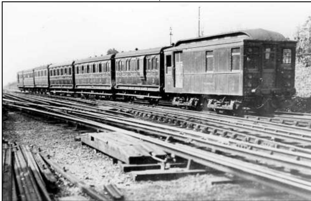
Fig. 7: A photo of a single District electric loco (believed to be 7A) with a train of old LTSR 4- and 6-wheel coaches. The destination plate shows “Pitsea”. The location is difficult to determine but I could guess that it’s possibly on the approach to either Acton Town or Barking. It could even be Ealing. It is recorded as being taken in 1925 by HGW Household.
