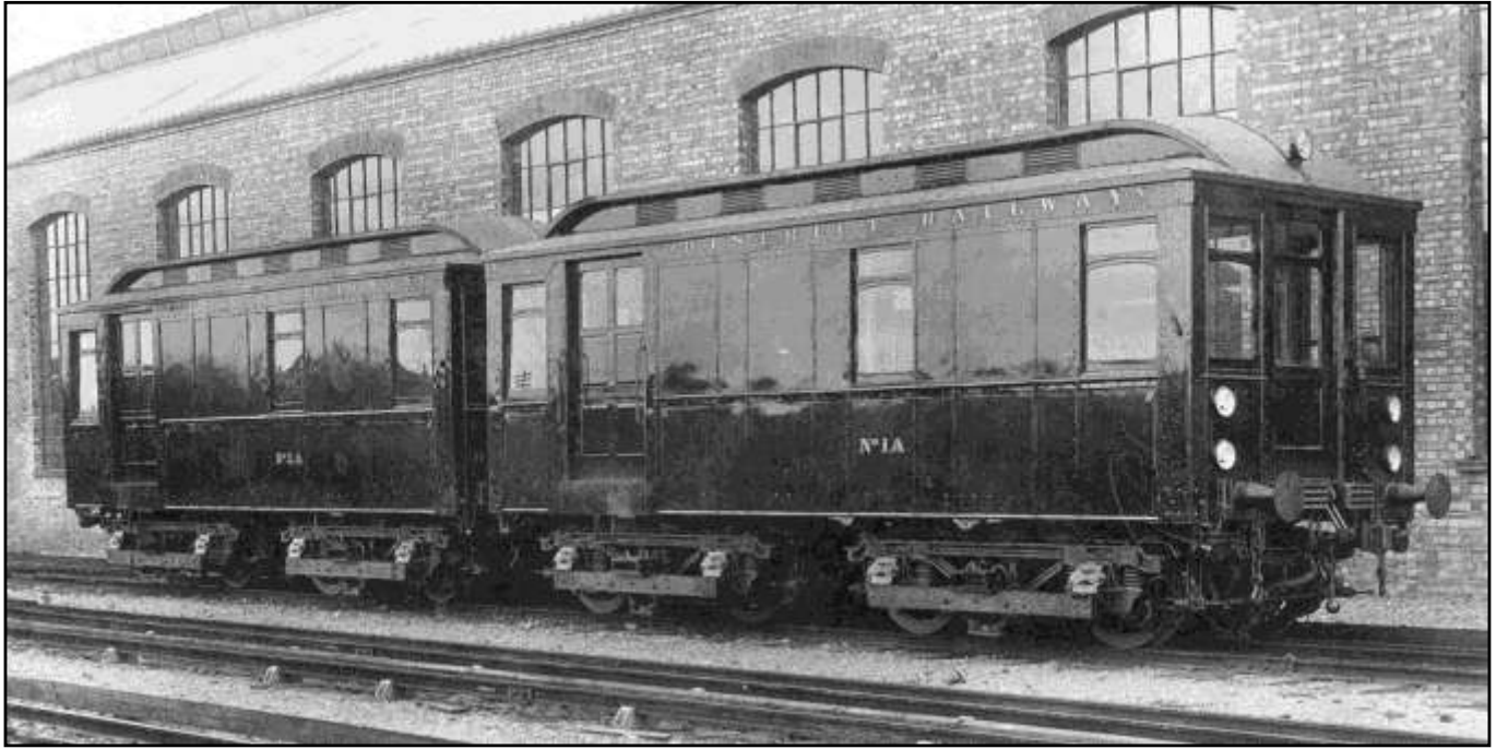
Fig. 1: A pair of District Railway electric locomotives, as new, standing coupled back to back outside the paint shop at Mill Hill Park depot (now Ealing Common). The bodies were mostly steel but they were similar in appearance to the wooden B Stock passenger vehicles. For operation with main line stock, side buffers and screw couplings were provided in addition to the standard Underground Ward couplers. The bodies were just long enough to allow two standard motor bogies to be fitted underneath. All other equipment was inside. I doubt the name DISTRICT RAILWAY lasted beyond the first overhaul.
